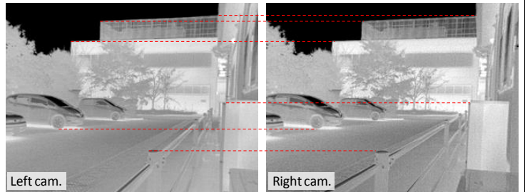
(b) Undistorted and rectified stereo image
